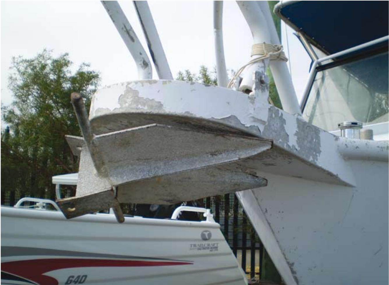
The metals don't have to be in physical contact but the solution such as saltwater transfers the current causing a reaction.
